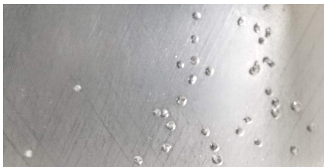
Figure 2. Pitting and bubble formation in can liners predict can failure by corrosion. Scale: 5 × 10 cm.
