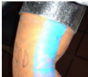
Damaged hose and tube covers.
