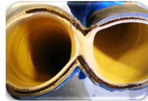
CIP caustic damage to hose reinforcement.
