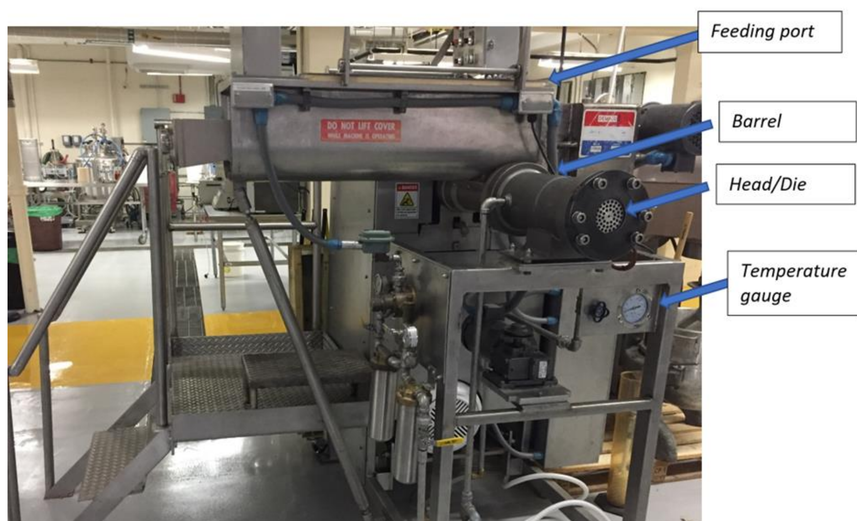
Figure 4. Diagram of extruder used to produce experimental aquafeeds
