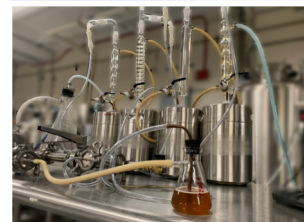
Figure 1: Vacuum fermentation vessels and sample collection chamber
