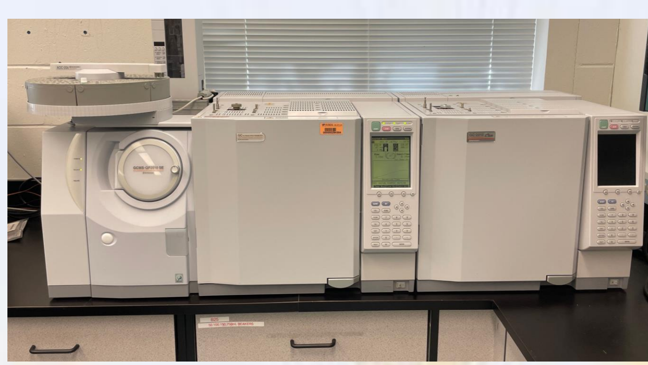
Figure 3. Shimadzu Gas Chromatograph (GC) 2010 plus series with mass spectrometer detector (MSD) used for volatile analysis of wort and beer samples.
